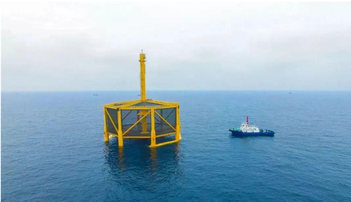
Figure 3 "Deep Blue 1," the world's largest fully submersible intelligent fishery aquaculture equipment independently developed by China (Image Source: xindemarinenews.com)
