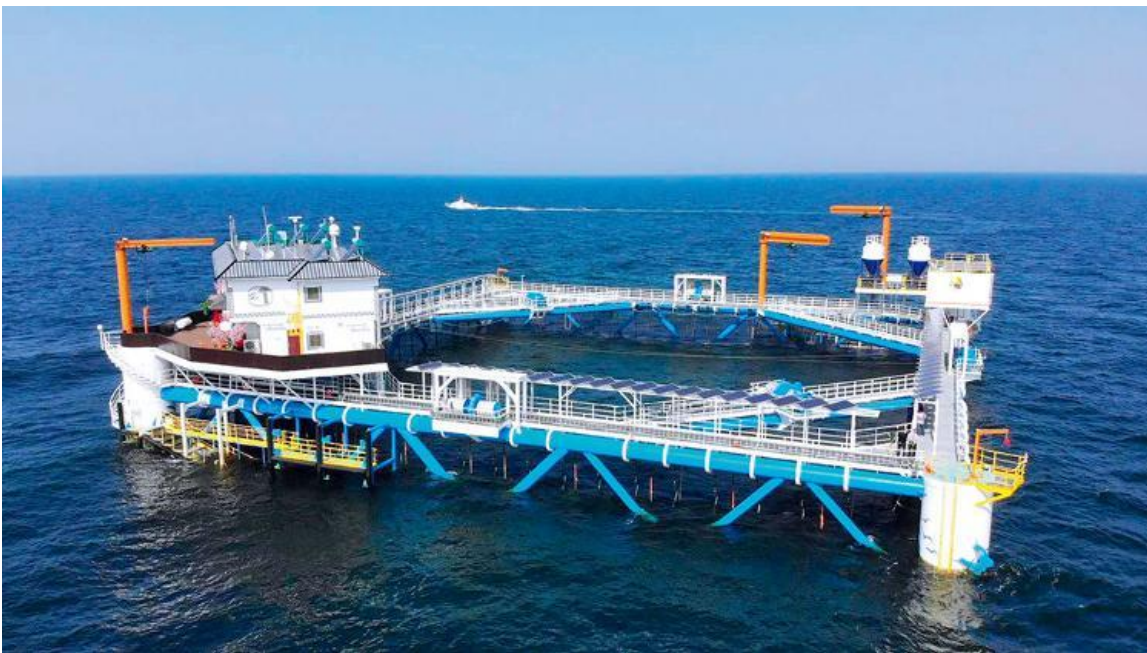
Figure 1 "Changqiong No.1" marine ranching platform in the sea area near Daqin Island, Shandong Long Island (Photo by Wang Kai)
